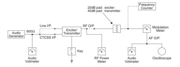
Figure 3.2 T826/827 Test Equipment Set-up
