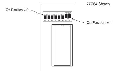
Figure 3.1 Channel DIP Switch Setting
